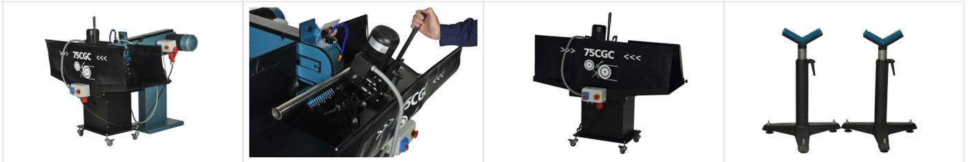
ARBOGA 75 CGC Centerless grinding and polishing machine is the perfect machine for polishing stainless pipes and tubes with its 2 speed motor and built-in coolant system.
