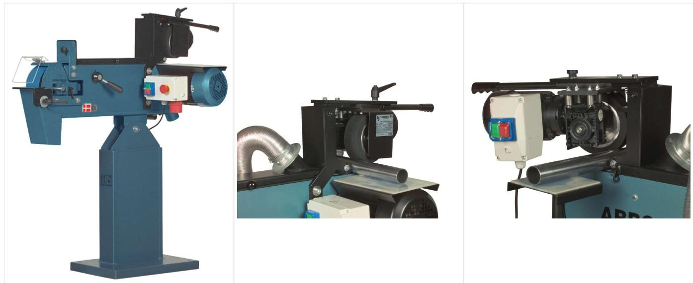
ARBOGA 75 CG centerless grinding and polishing machine is supplied with an attachment which can be mounted on all belt grinders with a 75x2000 mm belt and with a large grinding surface on top.
