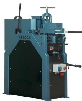
ARBOGA 150 RS pipe grinder is perfect for grinding all kinds of pipes and profiles before welding.
