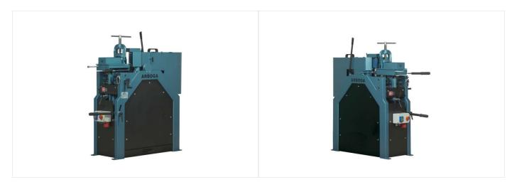
ARBOGA 150 RS pipe grinder is perfect for grinding all kinds of pipes and profiles before welding.
